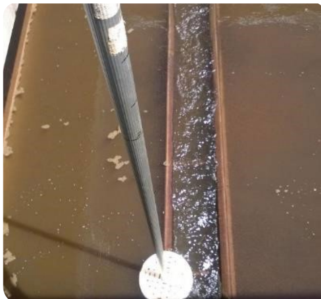
Figure 1. Modified Secchi disk used for filter assessments
