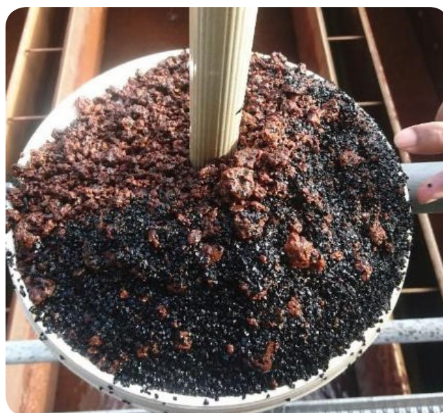
Figure 4. Examples of mudballs found during the final assessment. Note that although the amount has increased, the size is much smaller than previously observed
