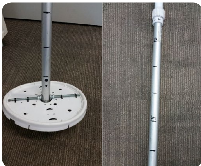
Figure 1. Detail of modified Secchi disk used for filter assessments
