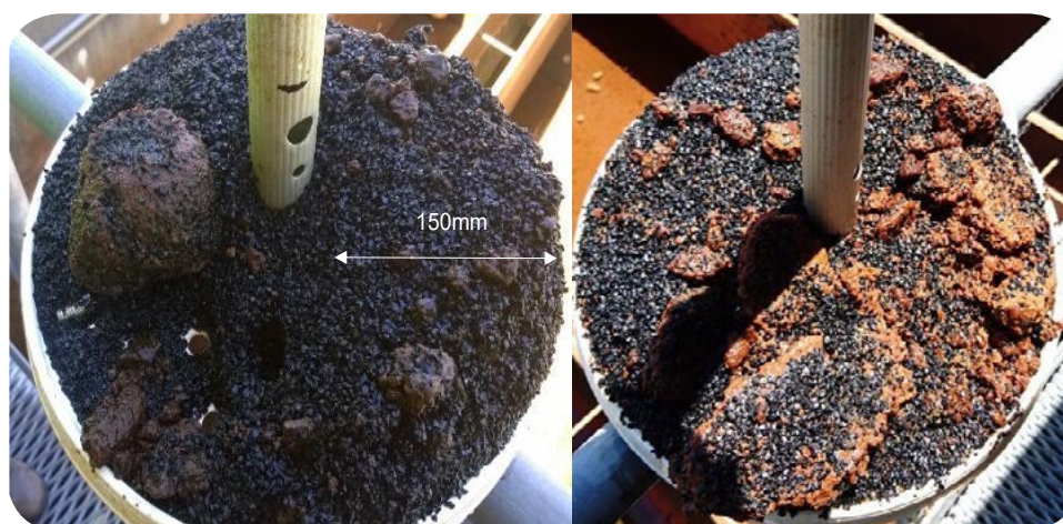
Figure 3. Examples of mudballs found during baseline testing collect after a backwash.
