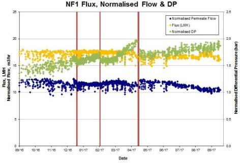
normalised DP has again risen at a slow rate and remains below the levels prior to the last CIP. On current trends each train should operate greater than 6 months before the next CIP is required.
