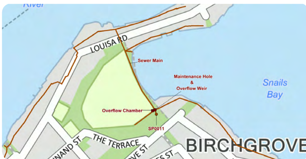
Figure 8. MapInfo layer marking the maintenance hole where SWI source detection monitoring was completed for SP0011. SewCam monitoring demonstrated that SWI was entering the sewer main from the overflow structure connected to the overflow chamber and underground stormwater during peak tides above 2.0m.
