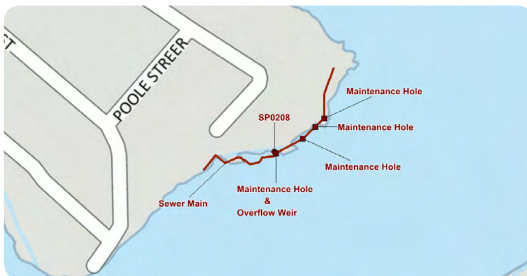
Figure 11. MapInfo layer marking the maintenance holes where SWI source detection monitoring was completed for SP0208. SewCam monitoring demonstrated that SWI is entering via damaged maintenance hole benching and isolated two sections of sewer mains north-east of SP0208.
