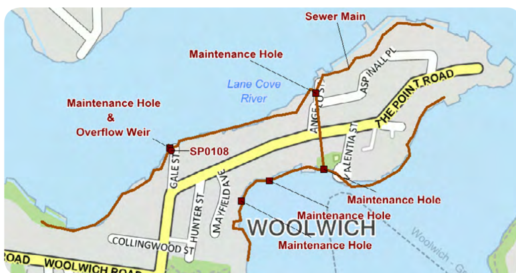
Figure 10. MapInfo layer marking the maintenance holes where SWI source detection monitoring was completed for SP0108. SewCam monitoring demonstrated that SWI is entering via the overflow weir, south-western and north-eastern sewer mains.
