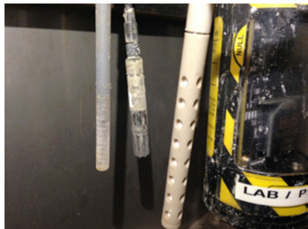
Figure 8. Sensors after 5 months in the sewer showing minimum biofouling (Left to right: Epoxy packaged sensor, conventional electrical sensor, PEEK packaged sensor, hydrogen sulphide sensor).
