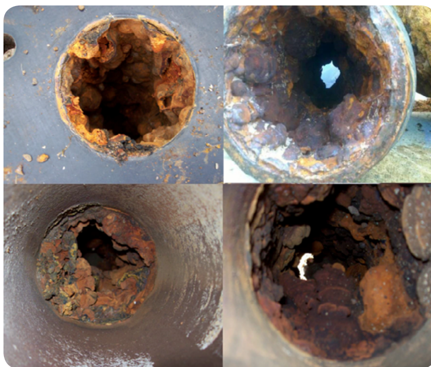
Figure 2. Tuberculation of unlined cast iron fittings
