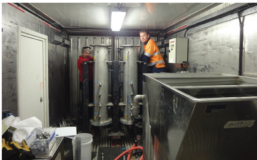
Figure 1. PRB installation to capture and treat hydrocarbon contamination from a diesel spill at Casey Station.
