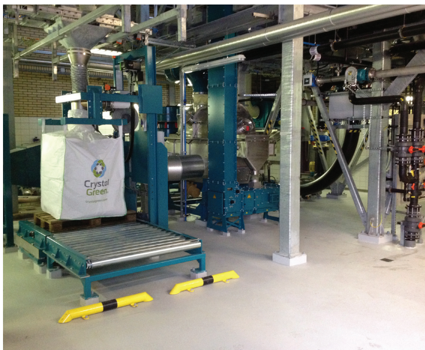
Figure 6. A bag of Crystal Green being filled from the Pearl reactor.
