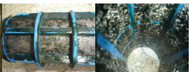
Figure 7. Screen filter after cleaning.
