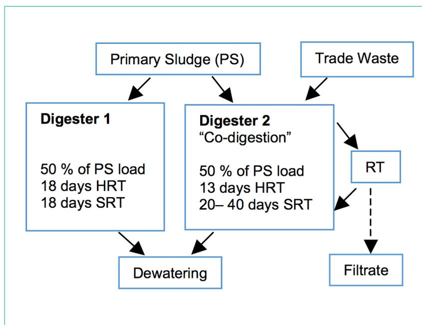
Figure 4. Process flow of the test plant.
