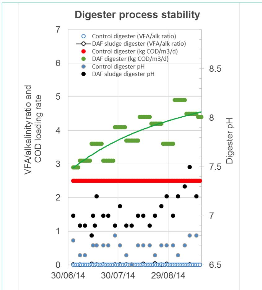
Figure 6. VFA/alkalinity ratio, pH and COD loading rate comparison in digesters D1 and D2.
