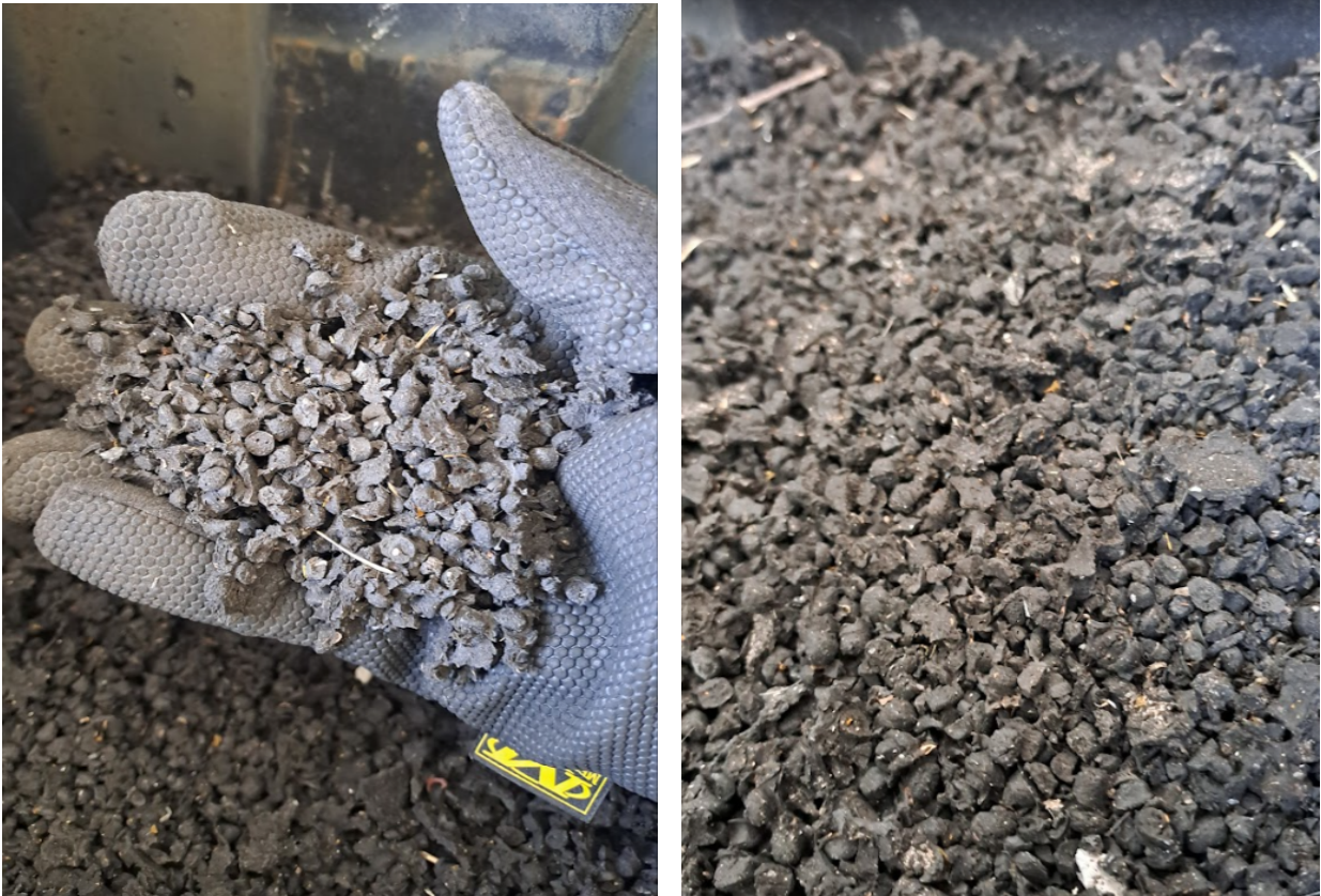
Figure 7: 3D-AeroDry®'s unique vertical sheet structure enables biosolids to form dried pellet-like materials during the drying process.
