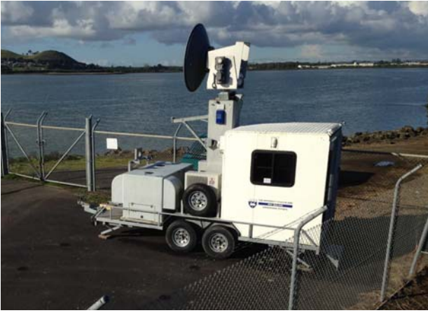
Figure 3: The University of Auckland high resolution rain radar overlooking the study catchment.
