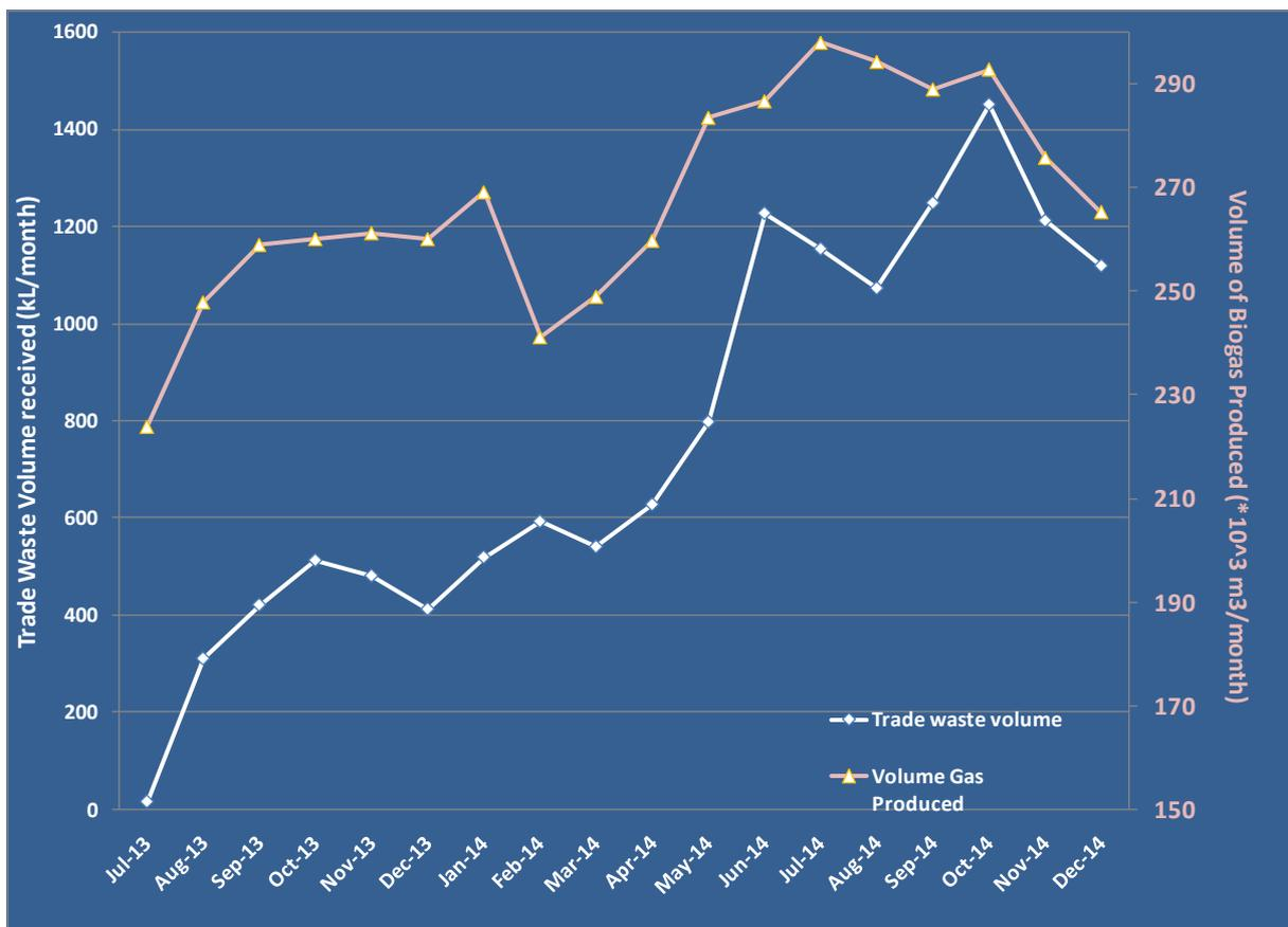
Figure 4: Volume of Biogas Produced and Trade waste volume received since the Co digestion plant commissioning
