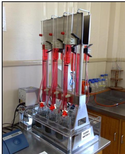
Figure 2: Eudiometer: small scale pilot plant to measure the biogas produced
